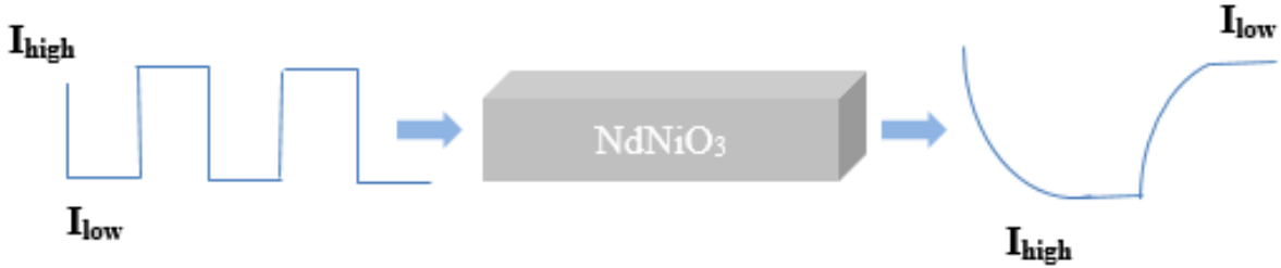
Figure 5.4 Schematic of two-level current-induced resistivity switching.
